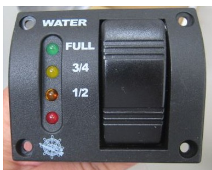
Figure 5: Water level indicator
